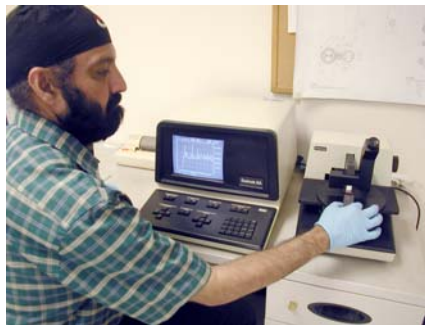
Vinder Jaggi measuring the thickness of a diamond-like carbon foil
