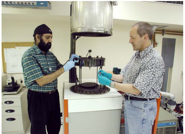
Vinder Jaggi and Stefan Zeisler examining carbon deposition slides used in foil production
